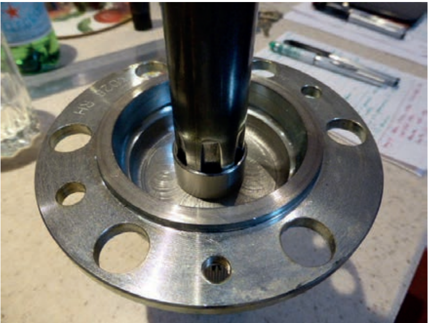
Rear hub with sleeve fitted
